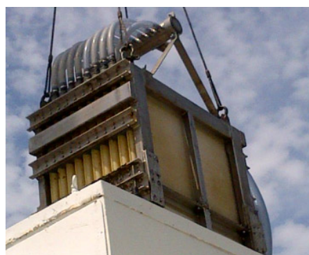
Figure 1: Membrane Bioreactor Example - Fibrecast FibrePlate (Fibrecast)
