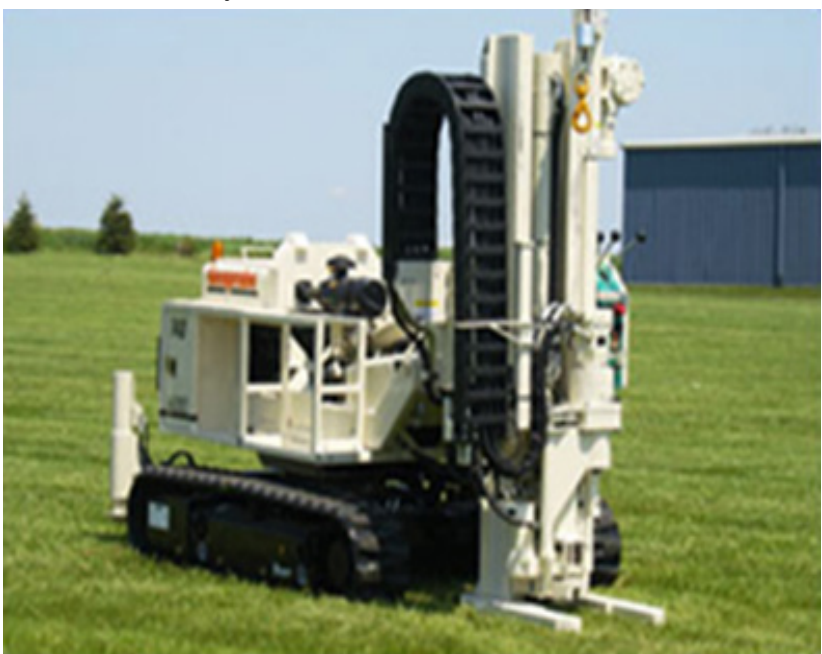
Figure 5 - Direct Injection Rig
