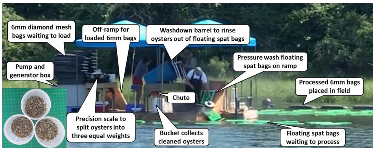
Figure 9. Floating Work Platform Configured for Splitting Y1 Oysters from Floating Spat Bags into 6 mm Diamond Mesh Bags
