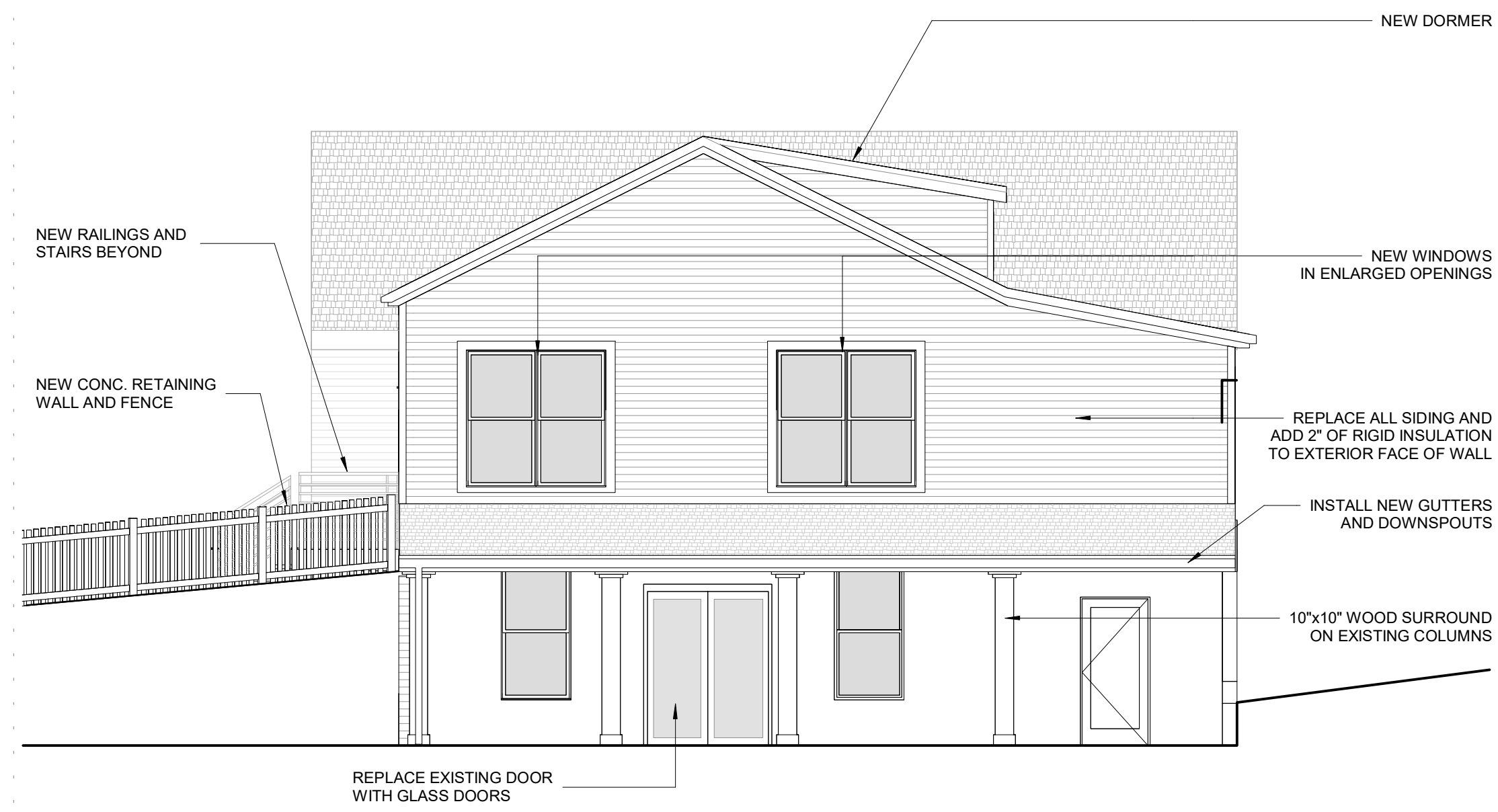
1 SOUTH ELEVATION - PROPOSED 3/16" = 1'-0"
