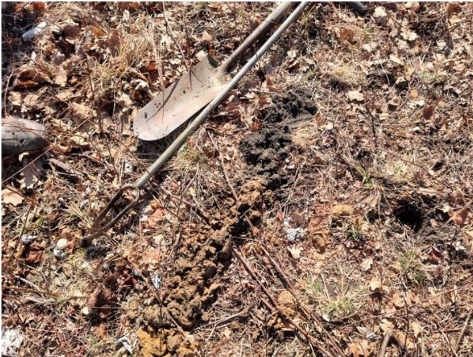
Soil test holes were dug to determine where wetlands had been filled. They were also useful in determining groundwater elevations, and soil texture by layer.
