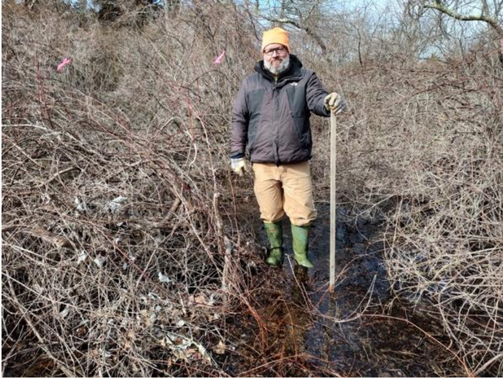
John Jannell places a wooden stake in the Shrub Swamp that will be used to monitor water levels and to serve as a benchmark for the elevations that were recorded.
