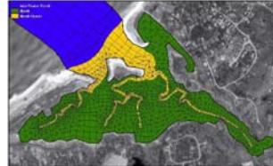
Plot of numerical grid used for hydrodynamic modeling of the Namskaket Creek system. Colored divisions indicate boundaries of different grid material types, as well as volumes used to compute flushing rates.
