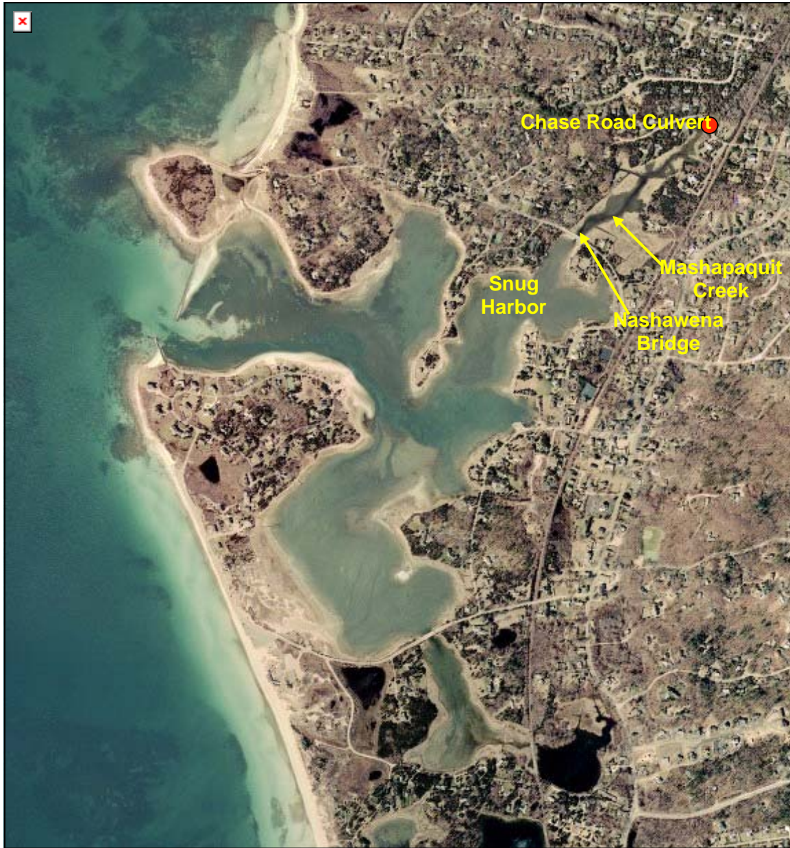
Figure IV-7. Location of Stream flow measurements (red circle) in the West Falmouth Harbor embayment system. Flow measurements obtained in Mashapaquit Creek at the Chase Road Culvert. Several studies of nitrogen transport from watershed source through Mashapaquit Creek prior to discharge to Snug Harbor support a removal rate of 40%.
