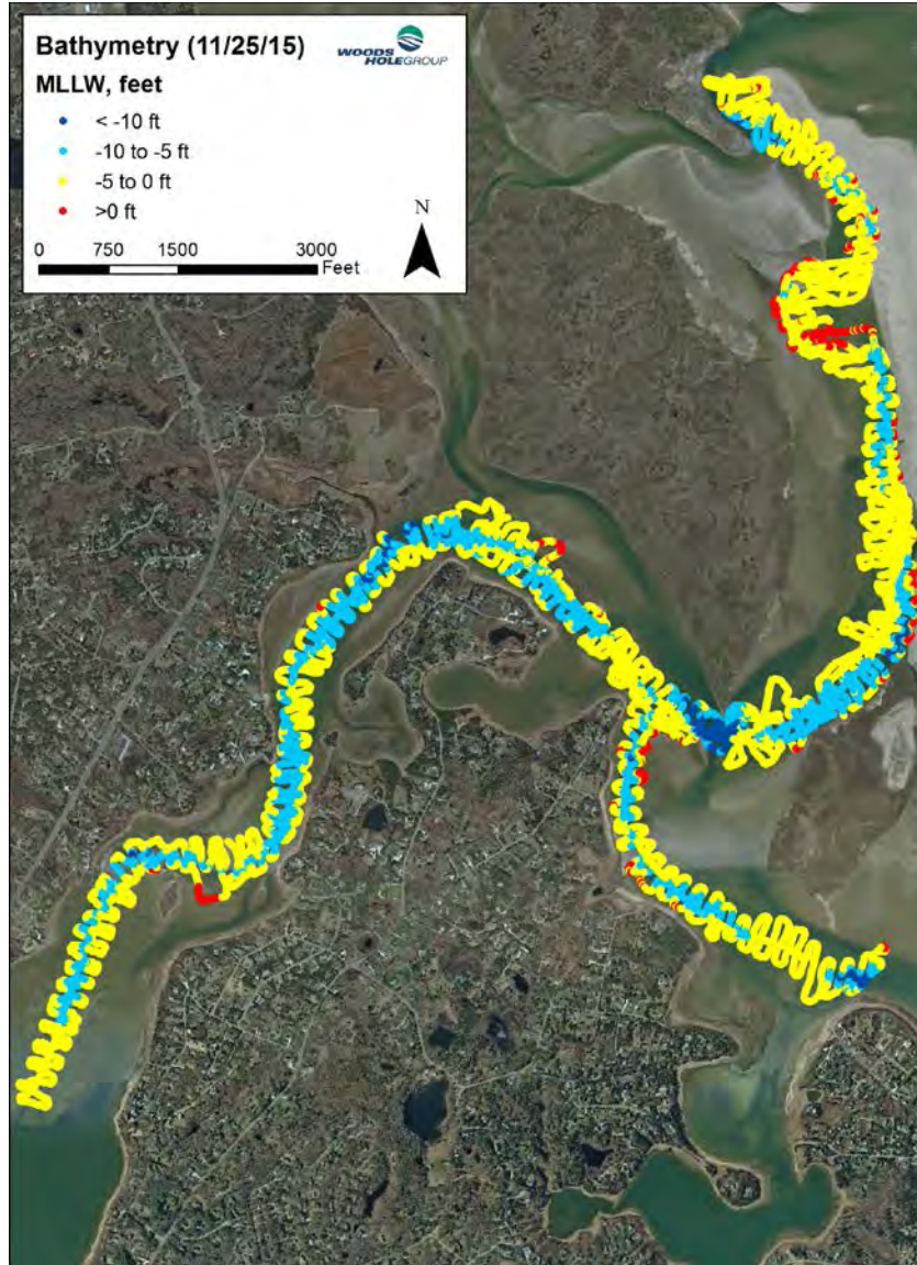
Figure 7. Color shaded map showing water depths referenced to MLLW from the November 2015 bathymetric survey.
